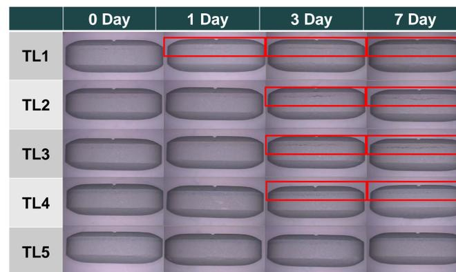
Figure 1. Delamination of the middle layer during the storage (40°C/75%RH without package) for 7 days.
