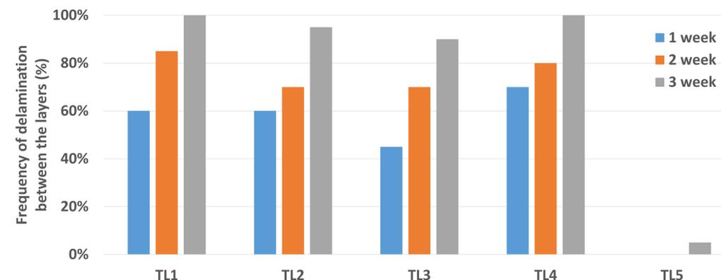
Figure 2. Frequency of delamination between the layers during the storage for 3 weeks.
